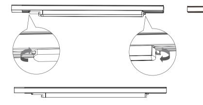
Rotate the clasp to ensure the light has been fixed with the track well. Adjust the rotary switch to the preferred circuit, turn on the power.
